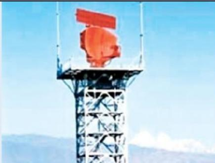
a secondary surveillance radar (SSR) that will give coverage of up to 200 nautical miles.
